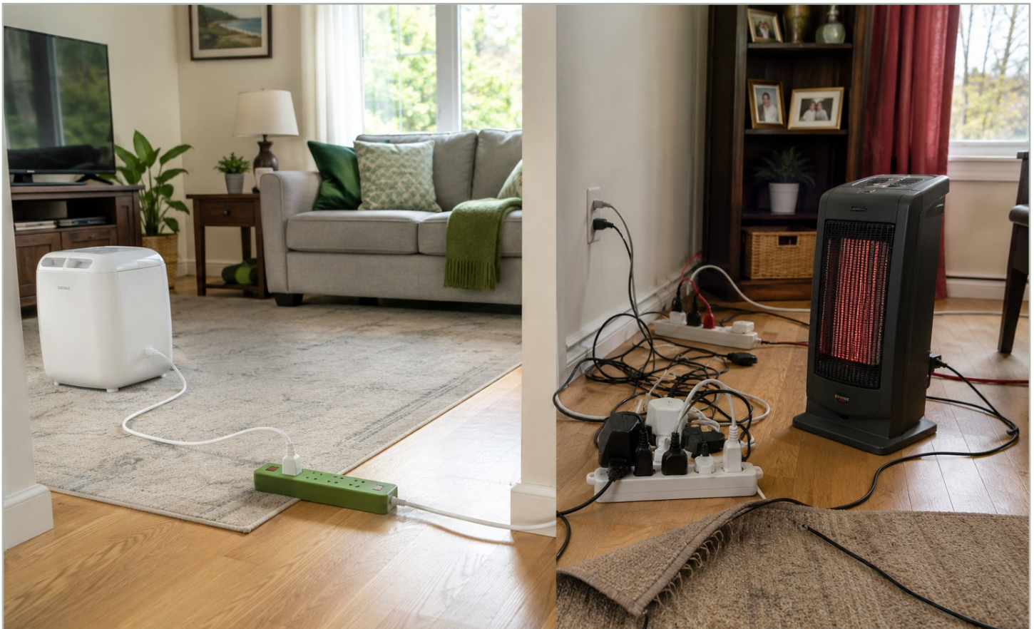
Safe temporary use on the left; overload and permanent-cord hazards on the right.
